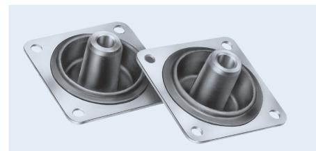
Barry Controls Multiaxis Mounts are designed for lowfrequency vibration isolation. These all-attitude isolators provide effective vibration protection in all directions and are available in either square or diamond configurations. Snubbing washers provide an interlocking system of metal fasteners which act to prevent damage from overload or excessive shock impact.
